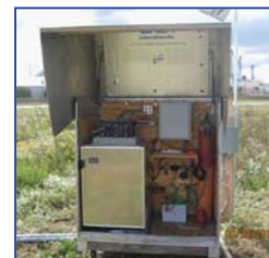
An inner look at one of the USGS gaging stations being used to monitor water quality at a field edge.
