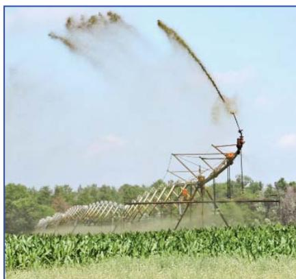
Center pivot irrigation equipment for aerial spray of untreated livestock manure.
