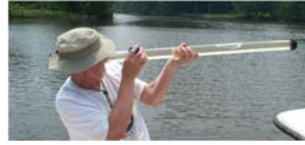
The Noel Morgan horizontal turbidity tube.
